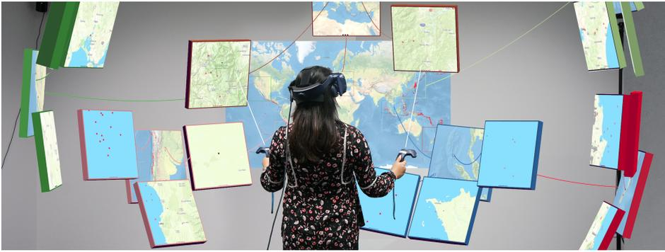
Fig. 1. Our immersive interface allows users to create large hierarchies of multiple maps at different scales and arrange them in 3D space. In the exploratory implementation shown here, a user views a spherical cap layout surrounding a large central overview. Visual links and colour hues indicate hierarchical groupings.
